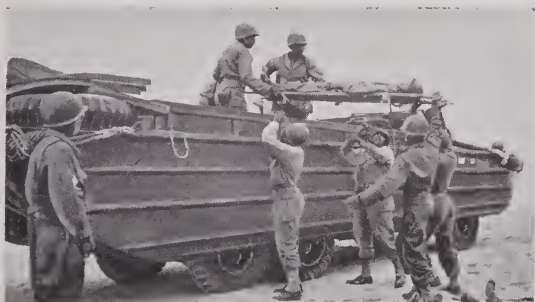
FIGURE 11. Passing up litters for top layer on DUKW. Handles of top litters can either be lashed with line or secured by plywood litter racks which are provided on all later DUKW models.
